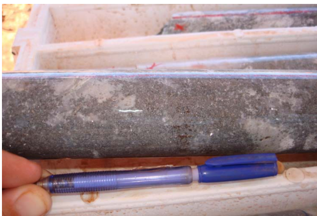
Two photographs of diamond core from Hole ARMCRCD001 showing sulphide mineralisation hosting gold, silver and copper. This hole was drilled 200m west of the main mineralisation at Mt Clement and represents a significant step-out discovery of a new zone of mineralisation.
